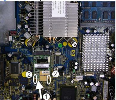
Figure 7-34 Removing the TV tuner module
